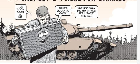
Mechanics, a little extra time when doing semiannual services on the M1-series tank's pulse jet system (PJS) will keep those V-pack air filters doing their job.
